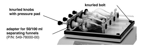
The adapter comes as an assembly. It is put on the shaker plate rubber cushion. Crimped edge of rubber plate is seated over adapter. Adapter is secured with 4 ea, knurled bolts located in the corners.
